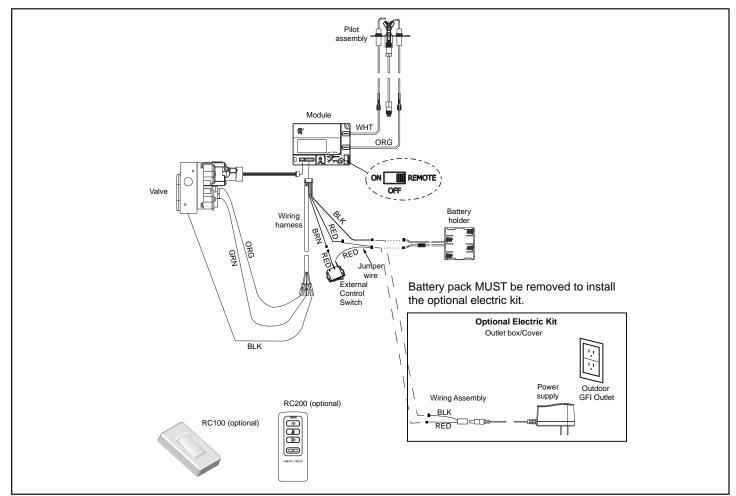
Figure 6.1 Intermittent Pilot Ignition (IPI) Wiring Diagram
